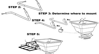
**STEP 3:** Determine whether to mount on the front or the back of the luggage rack. Depending on whether the M20 is mounted to the front or rear rack, you will need to install (#4) Control assembly to either the right (#11) or left (#15) Frame tube to allow for use with the non-throttle hand. Wait until the unit is mounted to the Quad before installing the Control.
